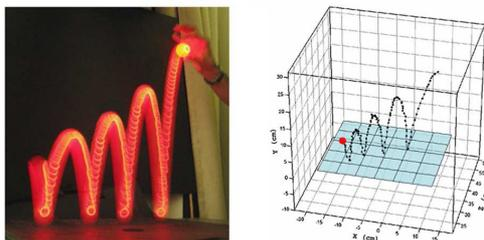
Figure 1: Real-time tracking of a pingpong ball.
