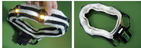
Fig. 3. The TR with its washable protective tissue, also showing the LED indicators (one per module). (Colours are visible in the online version of the article; http://dx.doi.org/10.3233/TAD-140414 )
