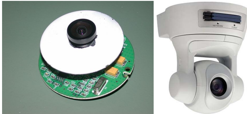
Fig. 2. Left: camera designed for flush mounting on surface. Right: a pan-tilt-zoom camera system.
