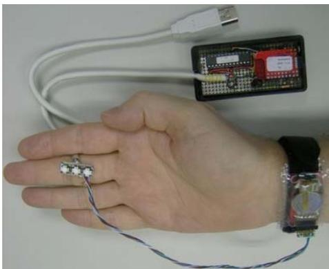
Figure 2: Magic Ring input device
